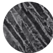
Cell structure – thermally modified timber
